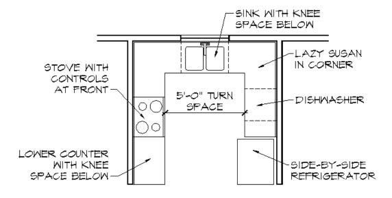
• Cabinets should be arranged around a 60" x 60" clear floor area, to allow a person in a wheelchair to turn around.
